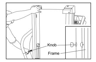
2. Hold the treadmill firmly with both hands, and lower the treadmill to the floor. To decrease the possibility of injury, bend your legs and keep your back straight.
